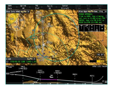
INAV<sup>™</sup> displays impediments and details of point to point flight, e.g.,
